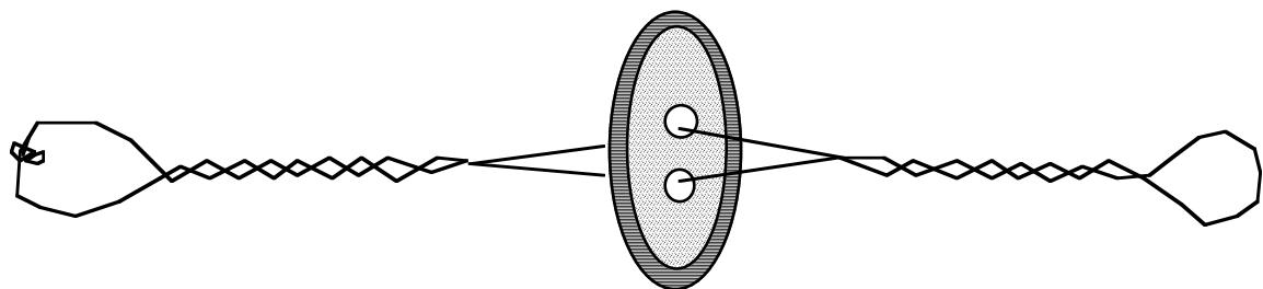
Buzzer made from a button and a loop of string
